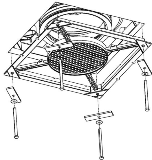
Figure 9- Assemble Bolt, washer & bar into duct & brace
